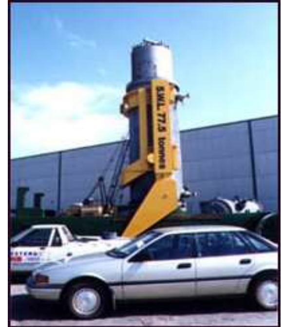
Catalyst Cooler Removal Unit
