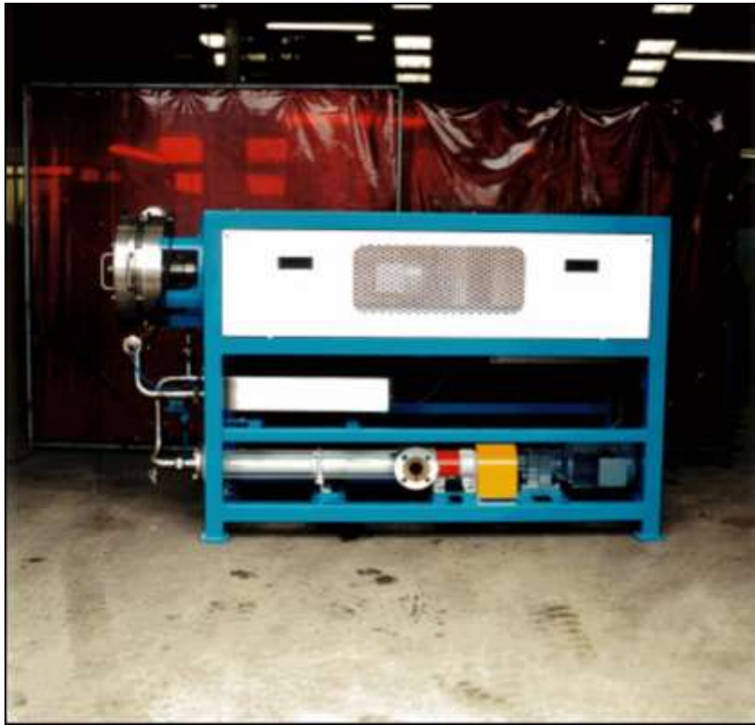
Foamer – used to deliver pre-cast latex to adhere tufted yarn to the backing media. The latex is foamed with air to reduce the volume of latex required so as to reduce cost
