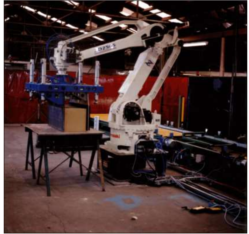
Tile Stacker – automatic conveyor system with robot to prevent manual handling issues and fingerprints
